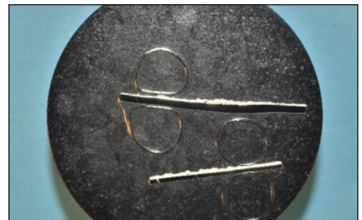
Metallographic mount containing cross-sections of the control and hail dent samples
